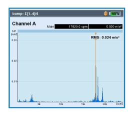
Bump Test to determine if the system structure has a natural frequency that interferes with pump frequencies
