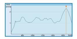
Ramp Up/Ramp Down test to determine at what speed the highest vibration occurs. This is an effective tool for VFD applications
